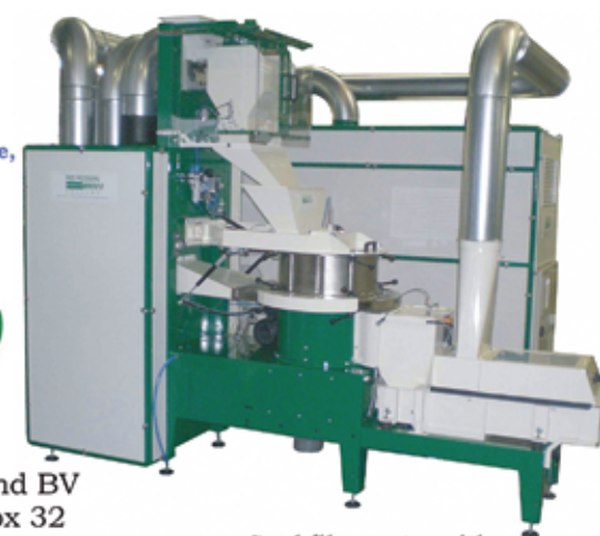
Seed film coater with integrated dryer
