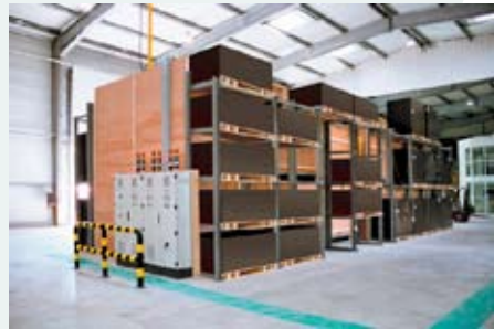
CONTINUOUS BOX DRYING INSTALLATION for drying each container/box individually
